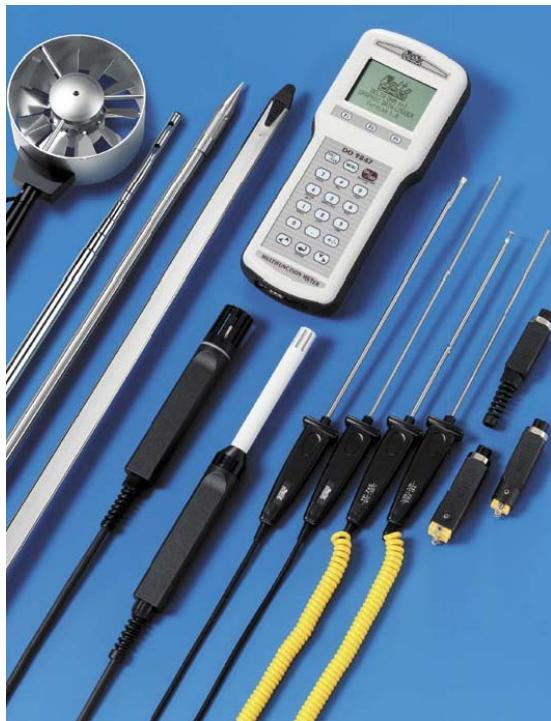
**DO9847** is a multifunctional handheld board instrument and datalogger. It is provided with a 128x64 pixel (56x38 mm) graphic display and three independent inputs. Each input can be connected to one channel or two channel dual probes (ex. two thermocouples, relative humidity /temperature, etc.).
