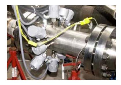
INLINE HEATER FLANGED as a source of hot air in a test
