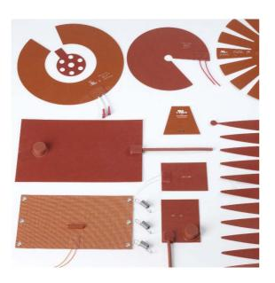
Silicone rubber is ideally su ited for the production of heater mats with it's low thermal mass and superb electrical insulation properties, it allows high power densities with fast response to temperature control. With silicones wide temperature range tolerance of -60°C to 230°C, being thin and lightwe ight it has a distinct advantage over other forms of heating elements. Where direct precise and intimate heating is required silicone heaters are the ideal solution.
