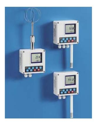
The devices of the HD2001 series..., according to the models, measure temperature, relative humidity, barometric pressure and, for the model HD2001.2, wind speed by hot-wire probes. All the models are provided with RS232C or RS485 serial output and the management of more than one device connected to a network. In addition, all the models are fitted with an open collector type low-activated configurable alarm output.
