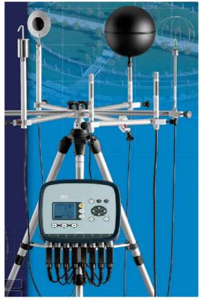
The Thermal Microclimate **HD32.1** instrument is manufactured by Delta Ohm Srl and it allows studying, measuring and controlling the Microclimate in the workplace, in compliance with the following standards:
