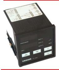
Din format 96x96 mm depth 78 mm.. Universal Microprocessor controller Programmable Input as Pt 100 Thermocouple (J,K,S) 0...20 mA, 4...20 mA. 0...10Vcc Range: depending on the input signal. Up to 3 output relays and voltage outputs for SSR or thyristor (0 .. 10V) RS 485 communication Chance Voltage 230V + 10% - 15% 48-62 Hz . 3,5 VA
