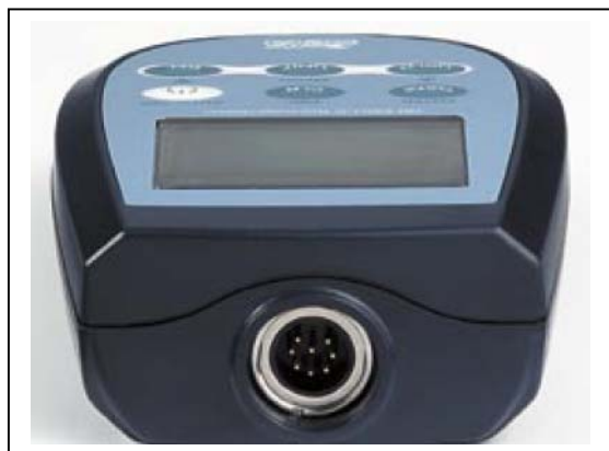
PP471 SICRAM Module Interface, between the probes and instrument
