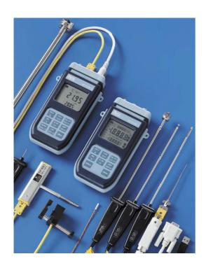
The **HD2108.1** and **HD2108.2** with one input and the **HD2128.1** and **HD2128.2** with **two** inputs are portable instruments with a large LCD display. They measure the temperature using immersion, penetration air or contact probes. The sensor may be a thermocouple of type K, J, T, N, R, S, B or E.
